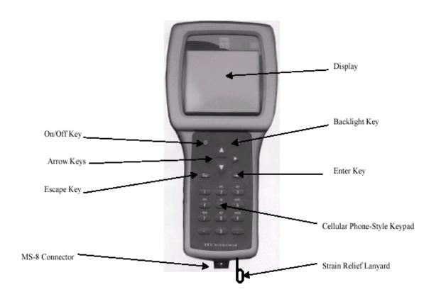
Note that the YSI 650 keypad consists of 20 keys as shown in the diagram above. There are four function keys, up, down, right and left arrow keys and an alpha/numeric keypad. The top left key that has a green circle and line, is the ON/OFF key. The top right key, activates the display backlight. The **Escape** key is labeled and is the **Enter** key.
