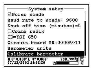
3. Press the **Enter** Key. Here you will have to know the outside barometric pressure in whichever standard you are using – typically mmHg. Enter the barometric pressure in the window similar to the one below. In order to ensure the most accurate reading, allow the handheld to adjust to outside temperature and pressure for a few minutes before taking the reading.
