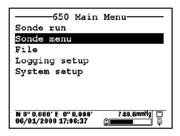
2. The handheld will make a sound that indicates that you are actively connecting to the sonde and its menus. Once connected, a screen like this will appear:
