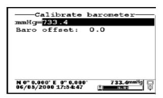
4. The screen below can be generated by entering the current pressure and pressing **Enter.** The offset value is used when returning it to factory settings. When you are finished, press the **Esc** button to return to the previous menu.
