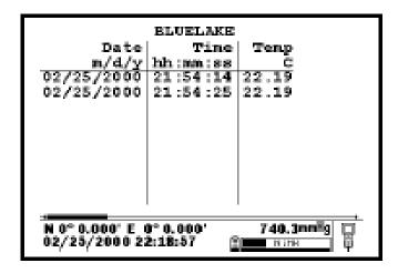
To view more data scroll over using the left and right arrow keys; to leave this menu, use the **Esc** key to move back. By clicking on **View File**, you will be able to view the any downloaded files and observe the values received from the river.
