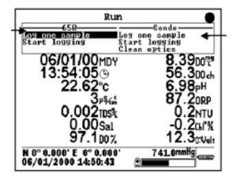
This screen shows all the parameters being measured. It may take a few minutes to settle to the river values being tested. Write or save the number. Exit the menu by pressing **Esc** and returning to the previous menu.
