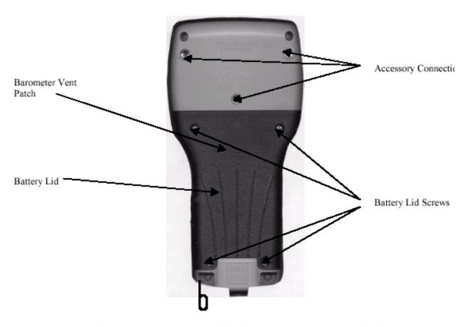
Note that the back of the case contains the battery lid that is attached to the main case with four captive screws and has three fittings for attachment of the ultraclamp and tripod accessories. In addition, the battery lid has a hole that is covered with water-impermeable patch for venting of the optional barometer.
