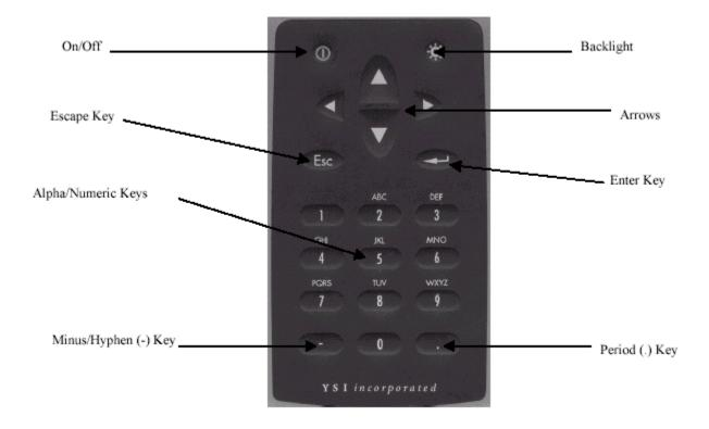
The **Enter** key always the user to proceed forward into other menus and screens. While the **Esc** key allows the user to move backwards through the menus and screens.
