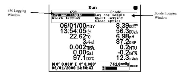
A screen will ask for a filename. Enter the name or number of the site being sampled on the keypad and press **Enter**. Next, using the right arrow on the directional keys, select **OK** and press **Enter**.
