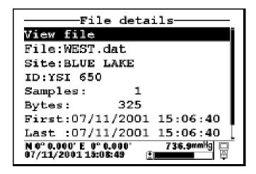
To see the values from the site select the words **View File** and press **Enter**. A new window with data such as date, time and temperature will be displayed as in the sample below.
