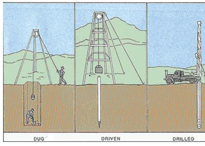
Driven wells are built by driving a small-diameter pipe into soft earth, such as sand or gravel. A screen is usually attached to the bottom of the pipe to filter out sand and other particles. They can only tap shallow water, and because the source of the water is so close to the surface, contamination from surface pollutants can occur.
