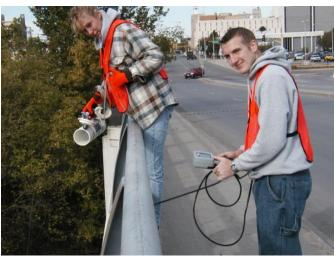
River Keepers uses a sonde and a sechi tube to get instant data from the river on pH, temperature, dissolved oxygen and others.
